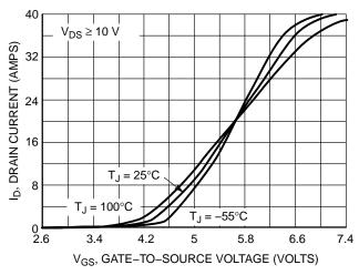
Figure 2. Transfer Characteristics
