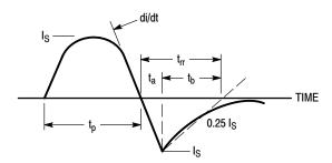
Figure 14. Diode Reverse Recovery Waveform
