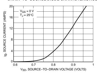
Figure 10. Diode Forward Voltage versus Current
